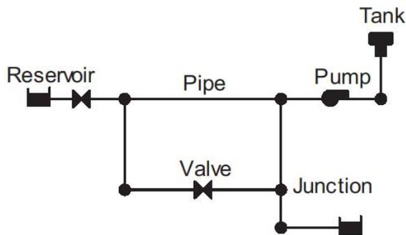
**Fig. 1** Components in a water supply system
