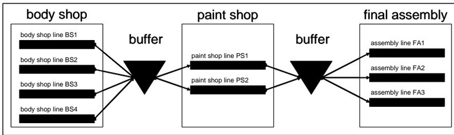
**Fig. 2:** General plant layout for car manufacturing
